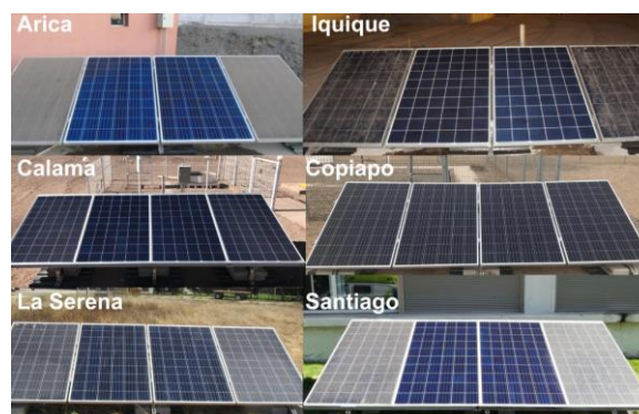
Figure 1. Photographs of the soiling measurement systems installed at deferent sites [12].
