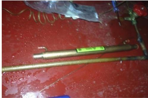
**Figure (5):** The Heat exchanger.
