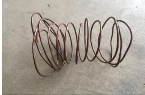
**Figure (3):** The Capillary tube.
