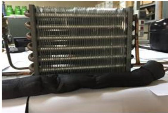
**Figure (4):** The Evaporators.
